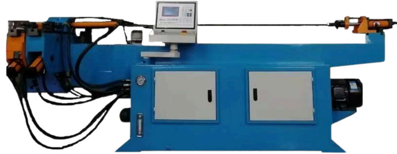
CNC PIPE BENDING-02
